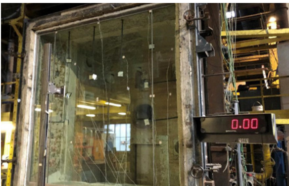
Fire resistance test
